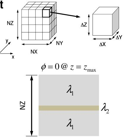
**<u>P3D</u>: Steady State 3D Heat Conduction by FVM (1/2)**  $\nabla \cdot (\lambda \nabla \phi) + f = 0$
