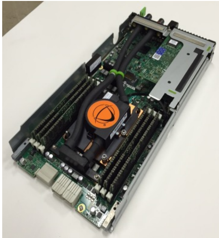
Computation node (Fujitsu PRIMERGY CX1640 M1) with single chip Intel Xeon Phi (Knights Landing, 3+TFLOPS) and Intel Omni-Path Architecture card (100Gbps)
