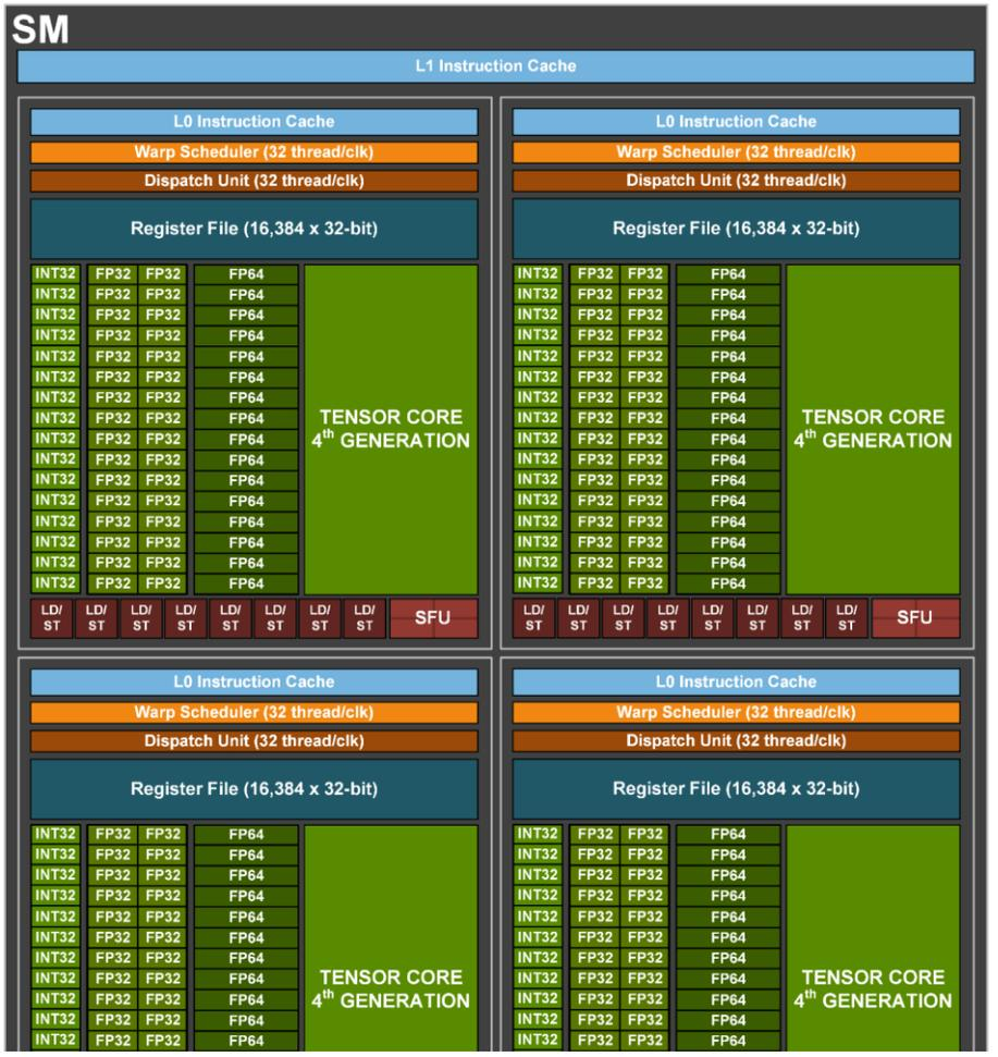
NVIDIA H100 Tensor Core GPU Architecture
