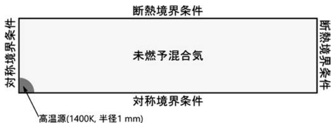
Fig. 2 A modeling of knocking combustion by using a two-dimensional constant volume reactor
