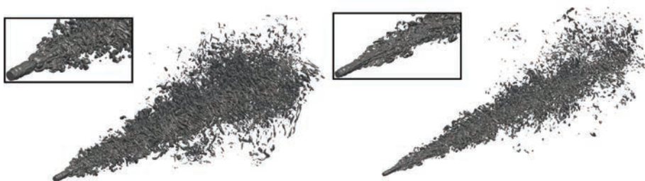
Figure 2: Effect of the diameter inlet reduction in the snapshots of the isosurface \alpha = 0.1 for cases 1 (left) and 3 (right). The details show the Kelvin-Helmholtz instabilities.
