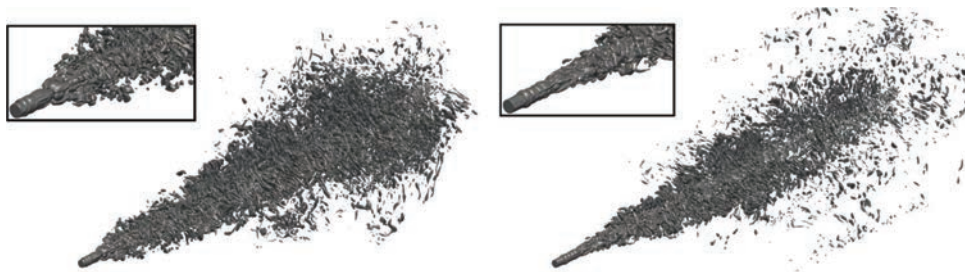
Figure 4: Effect of the density ratio reduction in the snapshots of the isosurface \alpha = 0.1 for cases 1 (left) and 8 (right). The details show the Kelvin-Helmholtz instabilities near the inlet.
