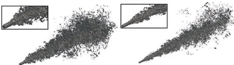
Figure 2: Effect of the diameter inlet reduction in the snapshots of the isosurface \alpha = 0.1 for cases 1 (left) and 3 (right). The details show the Kelvin-Helmholtz instabilities.
