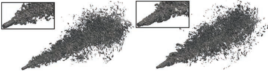
Figure 3: Effect of the viscosity ratio reduction in the snapshots of the isosurface \alpha = 0.1 for cases 1 (left) and 6 (right). The details show the Kelvin-Helmholtz instabilities near the inlet.
